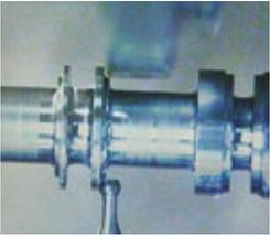
Our capability includes the ability to produce extremely precise close-fitting cylindrical components using technology developed from Moog Servo Valve manufacture. Typically we can achieve diametric fit tolerances of 1.25 micron and axial tolerances of 2.00 micron using our temperature control machining and measurement facilities.
