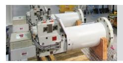
Once all the components are ready, highly skilled Moog trained technicians reassemble the actuators using authentic OEM parts including new seals, bearings, piston rods and body, and perform full load and performance testing.
