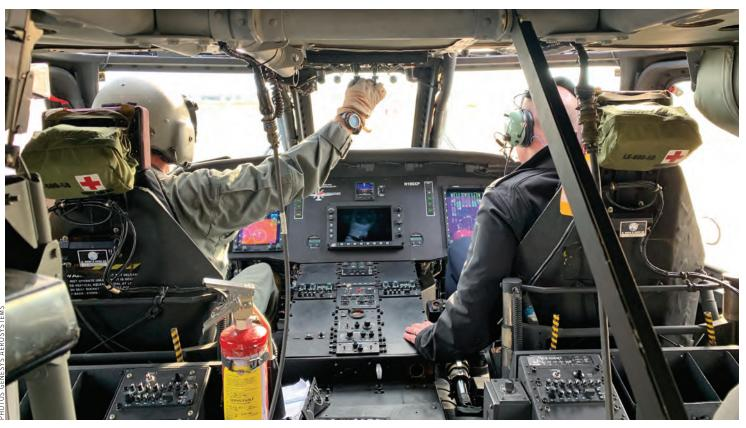
Genesys Aerosystems is upgrading Sikorsky UH-60 Black Hawk's with modern avionics and its HeliSAS autopilot.
