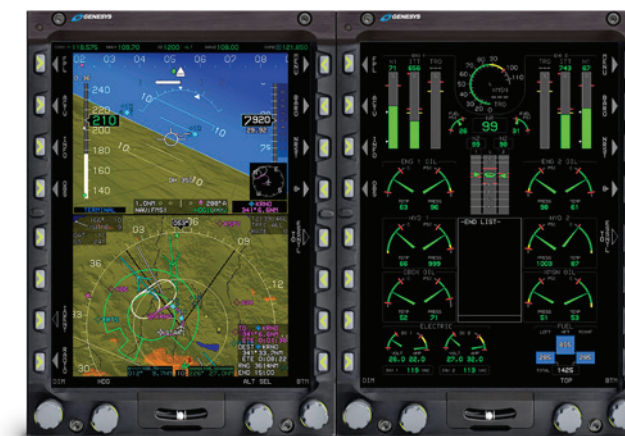
Genesys' multi-function display and the primary flight display view. The system offers pilots other views during various modes of flight.
