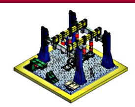
500 ton capacity 4 column portal frame for heavy duty vertical tests
