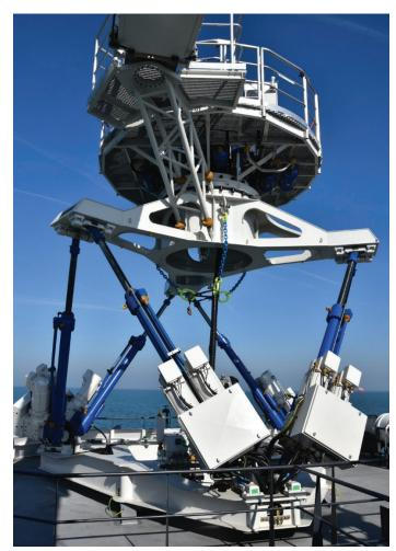
Fig. 1: New Ampelmann A-Type Gangway with EAS
