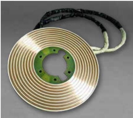
Fixed wing propeller aircraft use special de-icing slip rings to pass electrical power from the airframe generators to the rotating propellers. These propellers are heated to avoid the build up of ice either in flight or on the ground in difficult weather conditions.
