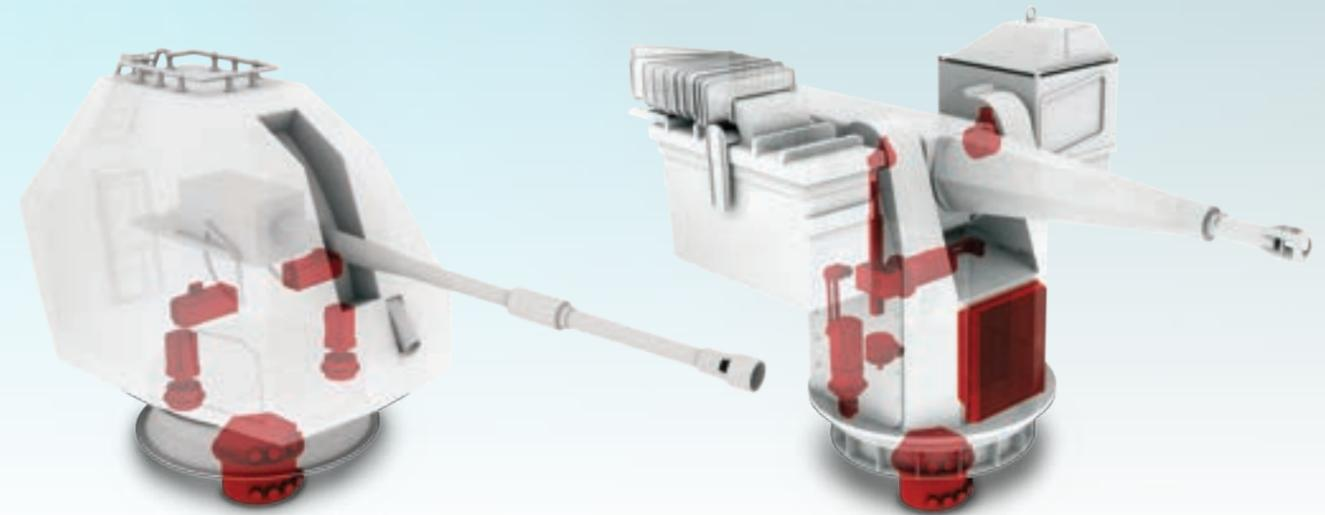
BAE Systems' Mark 8 Mod 1 naval gun: Moog provides the high performance motors for aiming stabilisation and ammunition loading. The slip ring transfers power and data.
